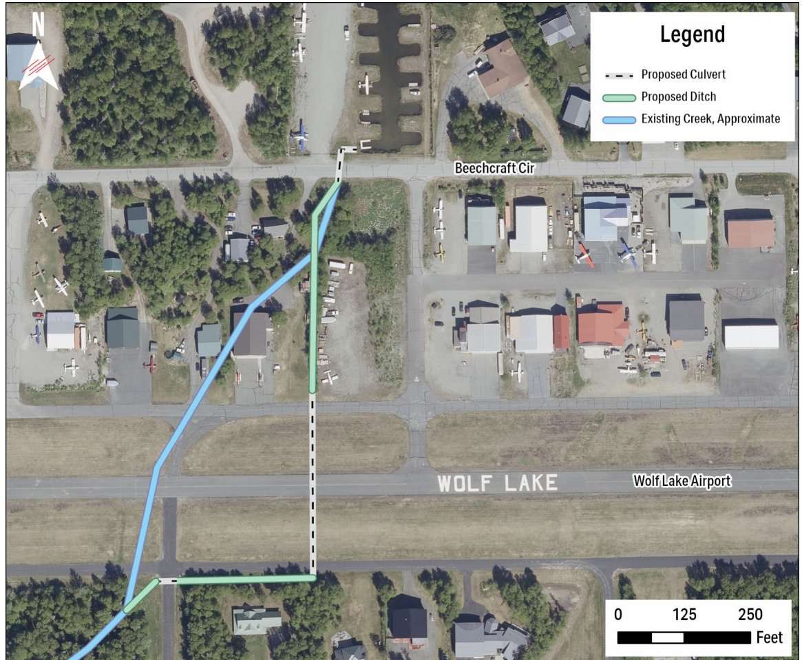
Figure 5-2. Wolf Lake Outlet Configurations
