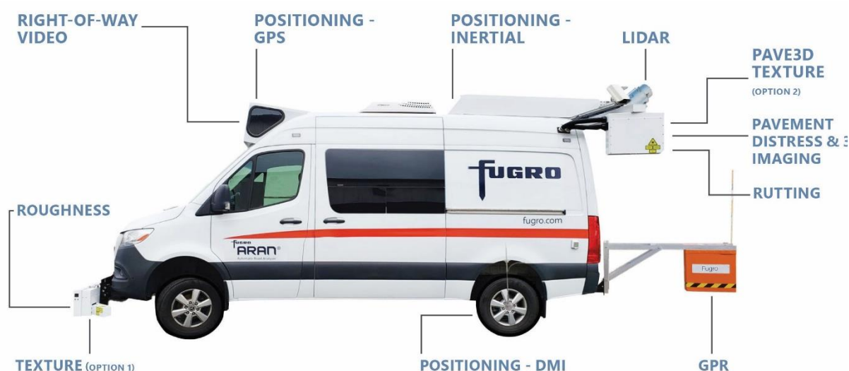
Figure 2.2: ARAN and its subsystems Set-up and field testing will utilize the exact same settings as the Alaska DOT project occurring at the same time. Weekly equipment controls will also occur under the jurisdiction of the State-level project
