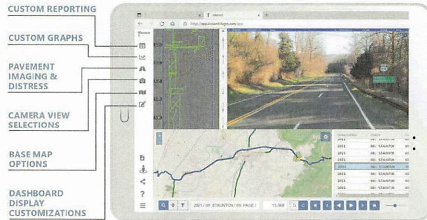
Figure 2.5: iVision5 navigation and inspection from a desktop or mobile device The web-app provides immediate access to all data streams places quality control (QC) ability right in the hands of Borough staff without the need of any additional IT resources
