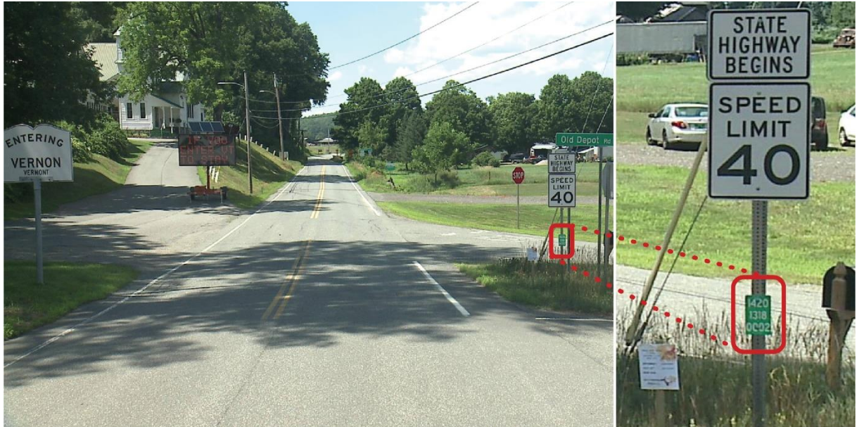
Figure 2.6: High quality imagery enables detailed asset extraction The photo demonstrates the quality of our ROW images, specifically in regard to asset extraction. The quality of the image allows the city staff ability to zoom into assets like road signs and review their condition from the safety of their desk.
