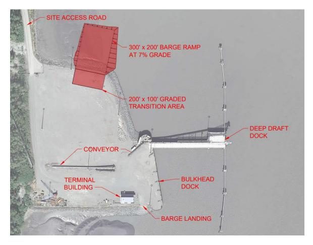
The results of the conceptual design study indicate that the project is feasible from construction, permitting, and operational standpoints. It is not anticipated that significant field efforts would be required to complete the design and permitting process. Permitting may be time-consuming and may take up to two years to complete. The OPCC for the recommended option is \$6,185,600.
